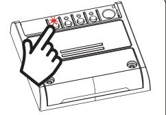
ACTION: Short press of button 1 during the Flashes LED: Turns off
