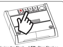
**ACTION:** Short pressure of button 2 during the Flash **LED:** Stop Flashes
