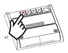
**ACTION:** Short press of button 1 **LED:** Flashing quickly and turns off
