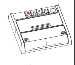
**ACTION:** Make a transmission with the transmitter **LED:** Flashing quickly and turns off
