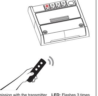
**ACTION:** Make a transmission with the transmitter **LED:** Flashes 3 times
