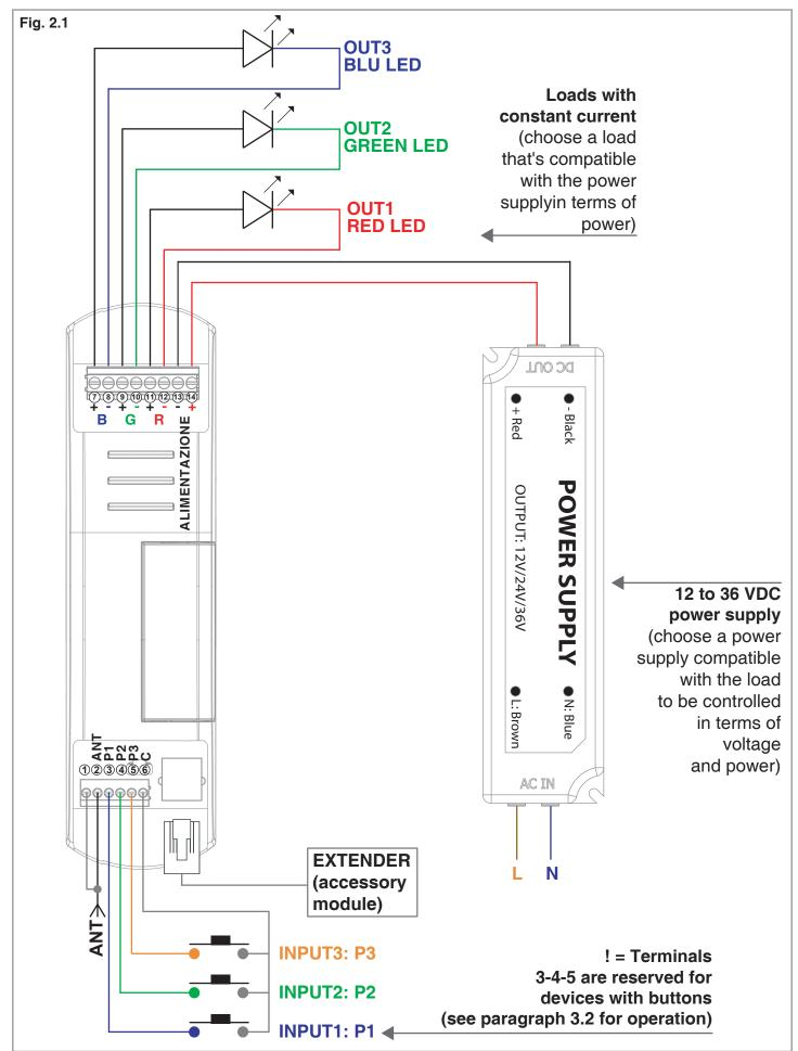
NOTE: multiple buttons or loads can be connected by using parallel cabling.
